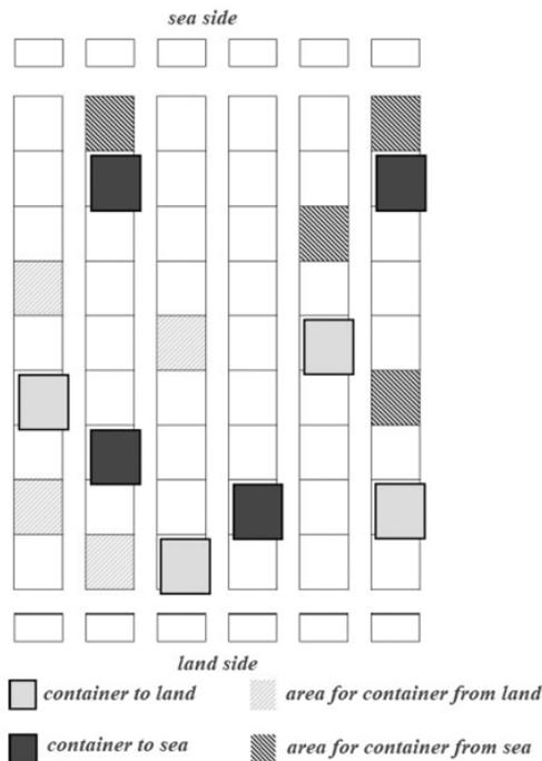
Figure 3: schematic representation of a stack block
