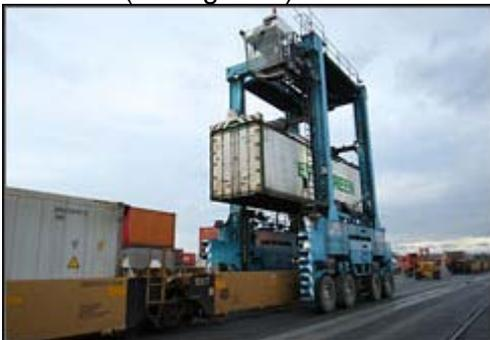
Figure 2: a straddle carrier at work
